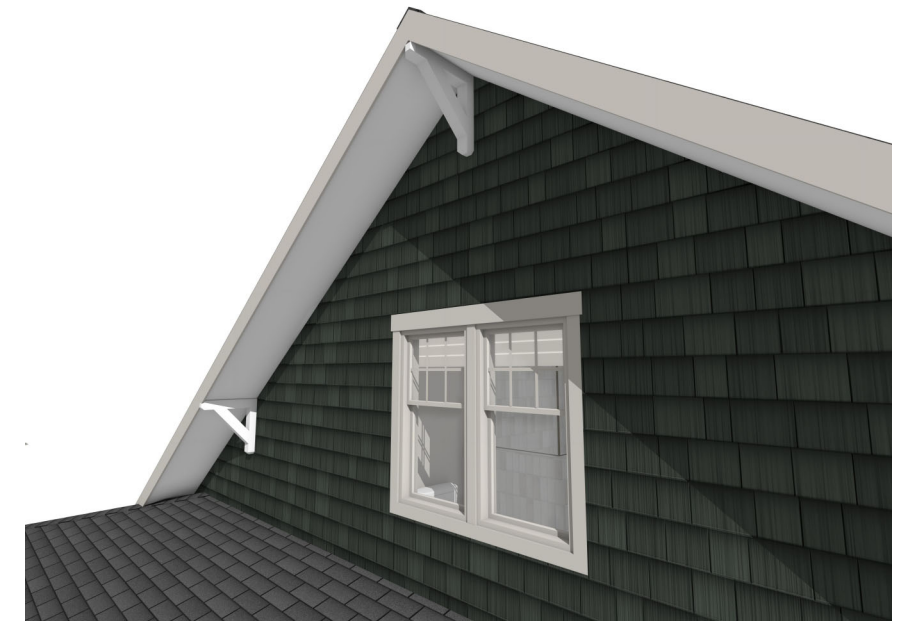
SHINGLES AND KNEE BRACES @ FRONT GABLE
